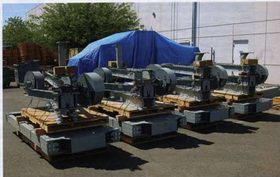
▲ Santos Fabrication, Turlock, Calif., fabricated counterweight and sling assemblies like these for the NASA Marshall Space Flight Center in Huntsville, Ala.
